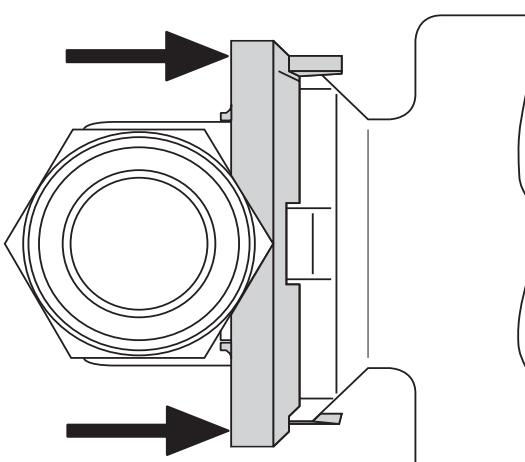
To release the metering unit, press the retaining ring towards the connecting module.
