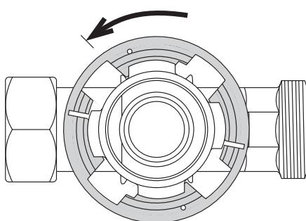
3. Use two hands to pull the blue retaining ring towards the device until it clicks into place. The device cannot be rotated unintentionally.
